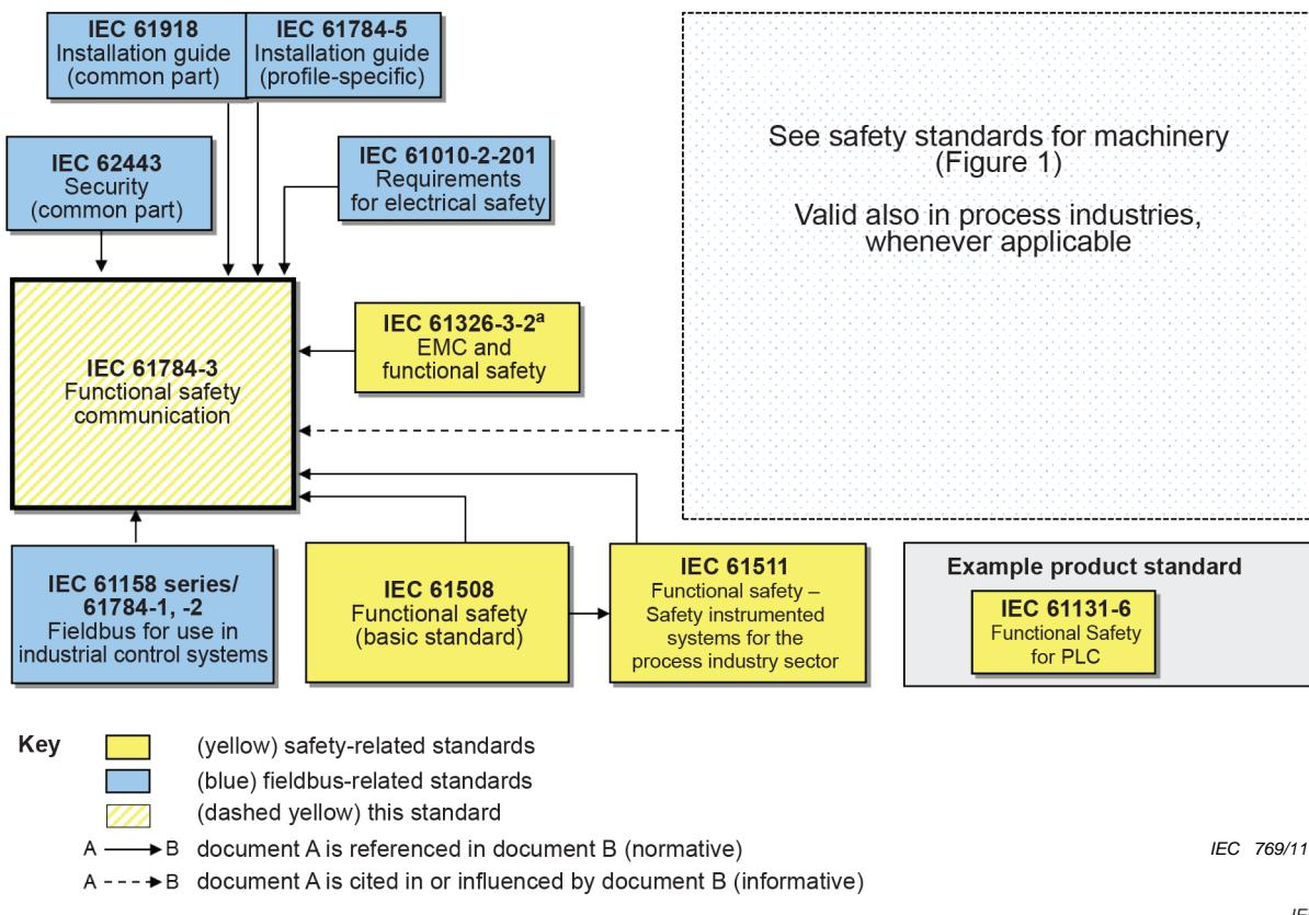
**Figure 2 – Relationships of IEC 61784-3 with other standards (process)**
